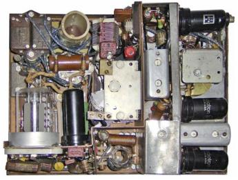
Bottom view of BP 4: receiver components right and transmitter left. The RF output valve is not an original type 829 but a later commercial version. (A new photo with a correct valve is in preparation)
